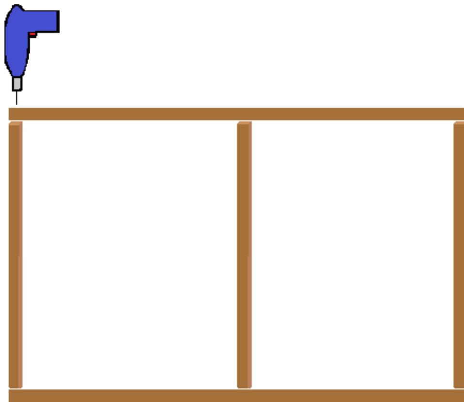
When you screw into a hardwood, the strips might separate, which isn't wanted. Remove the screw and try again until it is tight against the other wood segment. The second time should bring the boards tightly together because of the grooves made by the first attempt.
