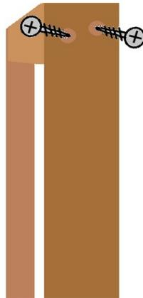
Afterward, a small 5/16 drill bit will be needed to drill a hole in the bottom of each crater so a screw can fit snugly inside. The pre-drilled hole is to keep your screws from breaking off, since using a hardwood can apply lots of stress on the screws when you are trying to put them in.
