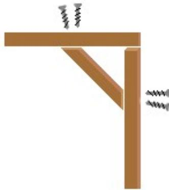
Like before, use the bevel drill bit to allow screw heads to sink in, and then pre-drill holes into it so the screws can easily go in. Do this for all four corners before switching out the bit again. When you screw in the brace and tighten it, make sure the brace is flush or below the face of your frame on the side that will have the canvas.
